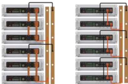
Figure 5-1 Schematic diagram of power cable connection
